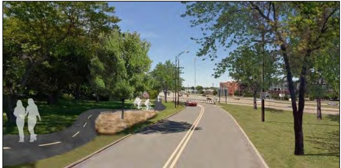
Top right: a stone wall and fencing treatment is proposed along the Yacht Club frontage. At a width of 8 feet, the path is less than the width of 10 feet recommended by AASHTO; a slight shift in roadway alignment could create the space needed for greater width, if desired. Below: trail along South Marginal Road.
